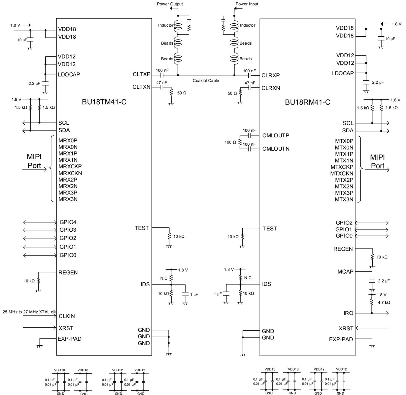
Figure 4. Applications Diagram (POC Cable)
