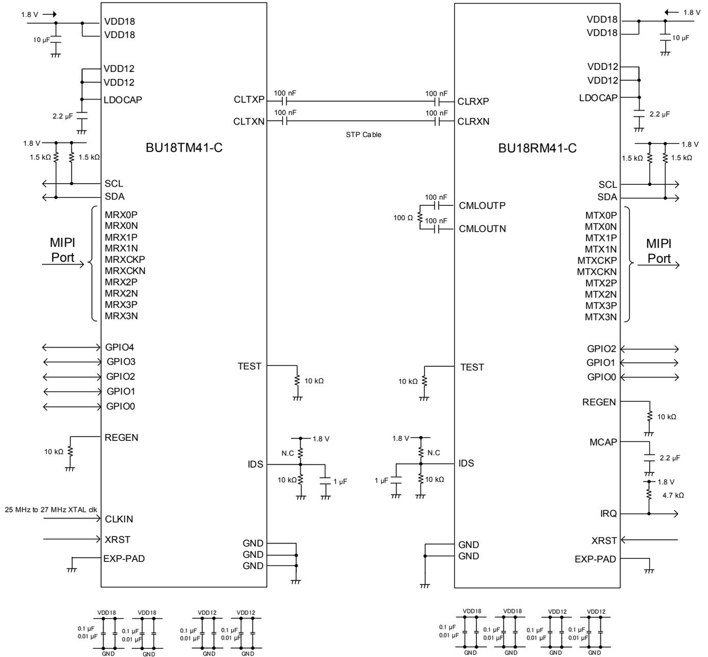
Figure 5. Applications Diagram (STP Cable)
